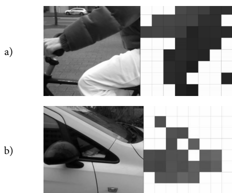
Figure 2. Two examples of what a normal webcam sees (top) and what the VL53L8CX sees (bottom). One of a cyclist (a) and one of a car (b), both at close distance
