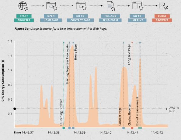
Figure 3b: CPU Energy Consumption in Joule over Time for User Interaction with Web Page as shown in 3a.
